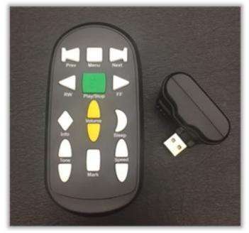
Figure 1- Remote control on left and IR receiver on right
